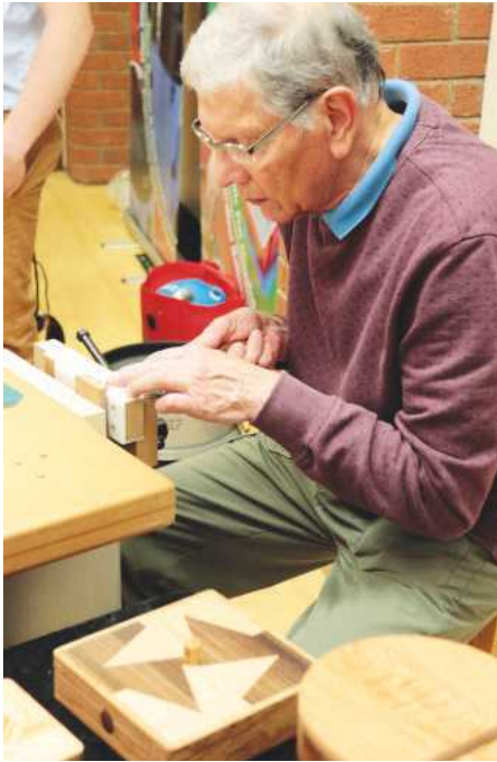
The second jig allows for the base of the tails to be quickly pared away from one side
